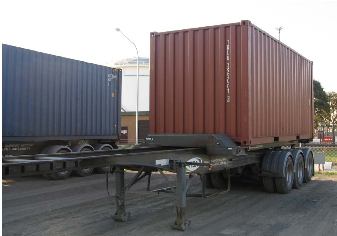
Figure G.7 Roll-back B-Double 'A' trailer with 20ft Container in Rolled Back Position
