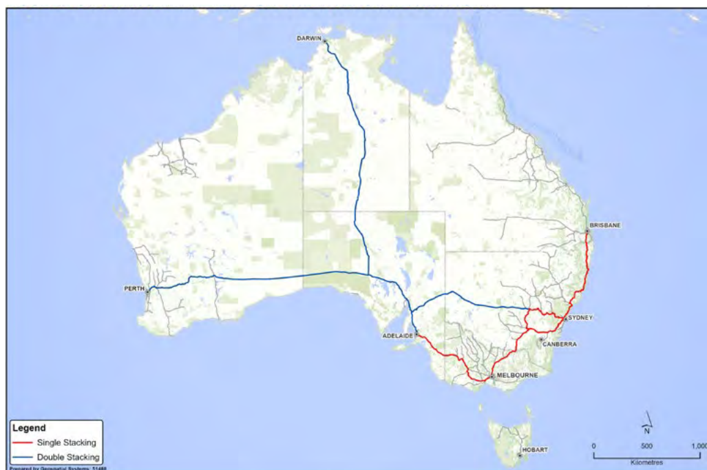
Figure 52 Double stacking capability on the interstate network
