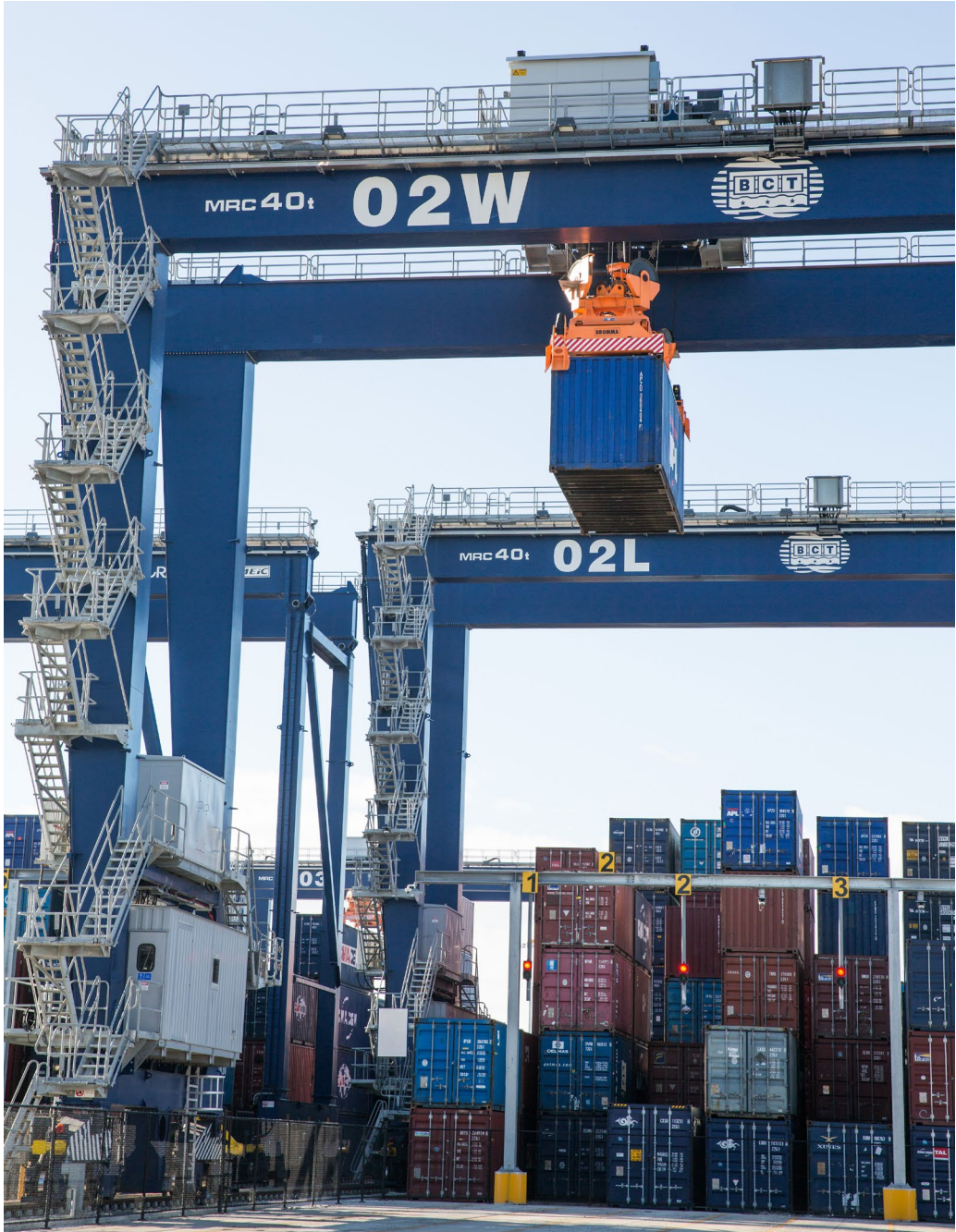
Brisbane Container Terminals Automated Stacking Crane, Port of Brisbane. Photo courtesy of Port of Brisbane Pty Ltd.
